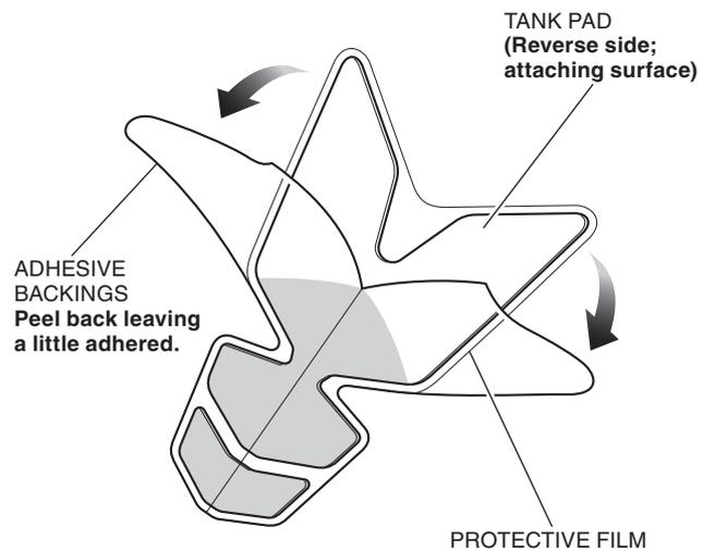
3. Loosely install the tank pad as shown.
