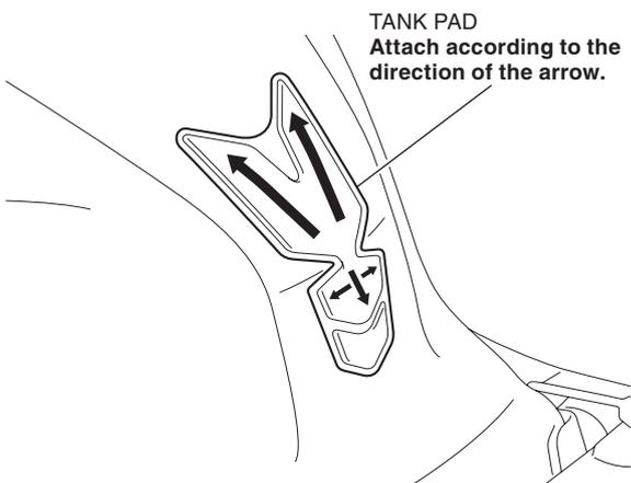
6. Apply adequate pressure to the attached tank pad and remove the protective film.
