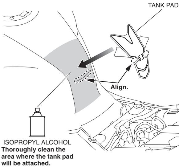
4. Attach the tank pad as shown.
